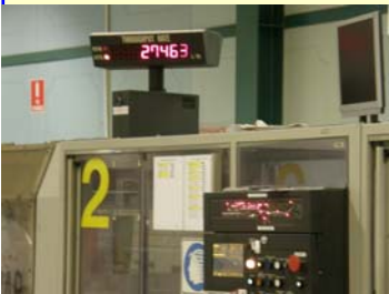
This is the special section for your mail if you forget to write the postcode on your envelope or package. The machine photographs the address and identifies the correct postcode
