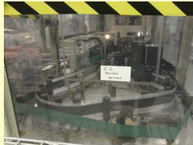
This is the special section for your mail if you forget to write the postcode on your envelope or package. The machine photographs the address and identifies the correct postcode
