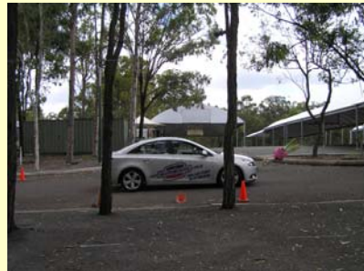
What would happen to a child running onto a road while vehicle travelling at 60km/h. The car hit the dummy at 30km/h
